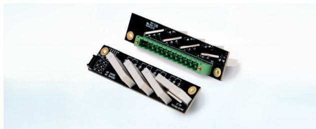
As an alternative to our AutoZero module, an interface card with three potential-free changeover contacts can also be integrated, which enables the operation of an external calibration device. Using this interface card, a zero gas valve and a calibration gas valve can be controlled independently of each other.
